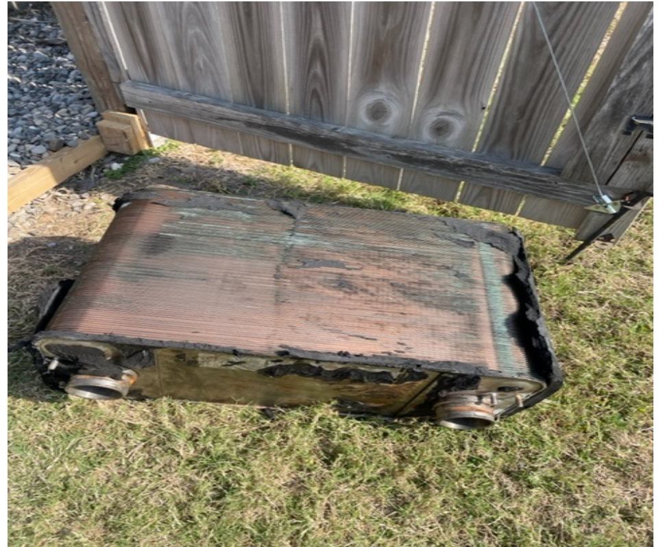
NON OPERATIONAL HEAT EXCHANGER
