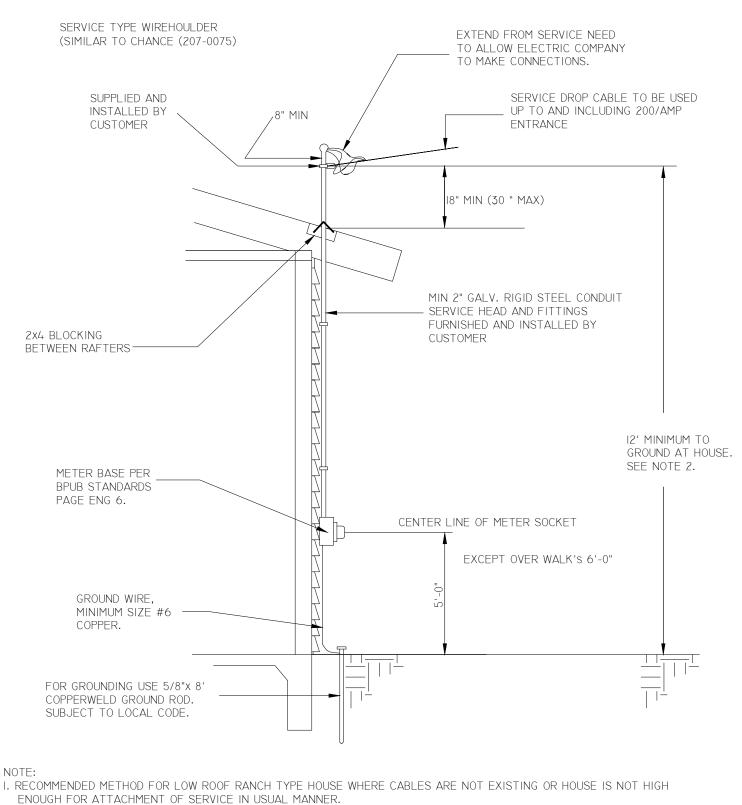
2. POINT OF ATTACHMENT FOR SERVICE MUST BE OF SUFFCIENT HEIGHT TO MAINTAIN, FOR THE SERVICE, A 12' MINIMUM CLEARANCE, 18' MINIMUM TO COMMERCIAL DRIVEWAY AND 22' MINIMUM TO STREET.
