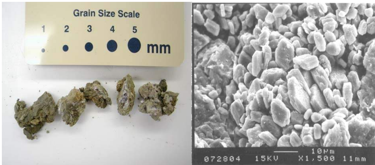
Figure 8: (a) Large grain gypsum crystals (b) Small grain gypsum crystals
